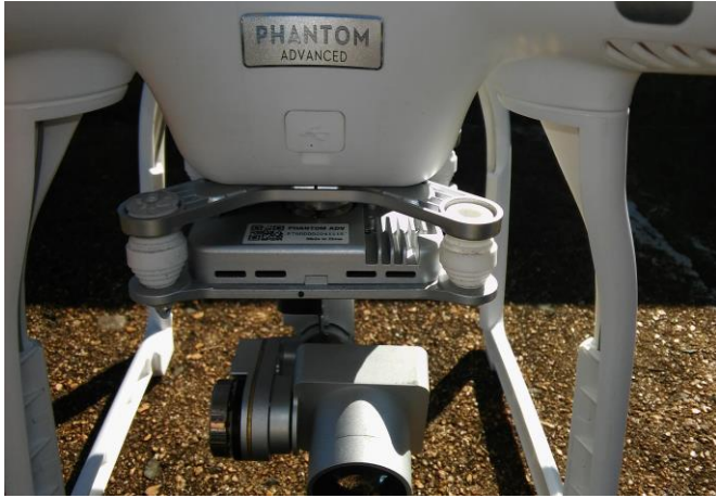
Figure 8: Phantom 3 drone camera with a stabilization mechanism.
